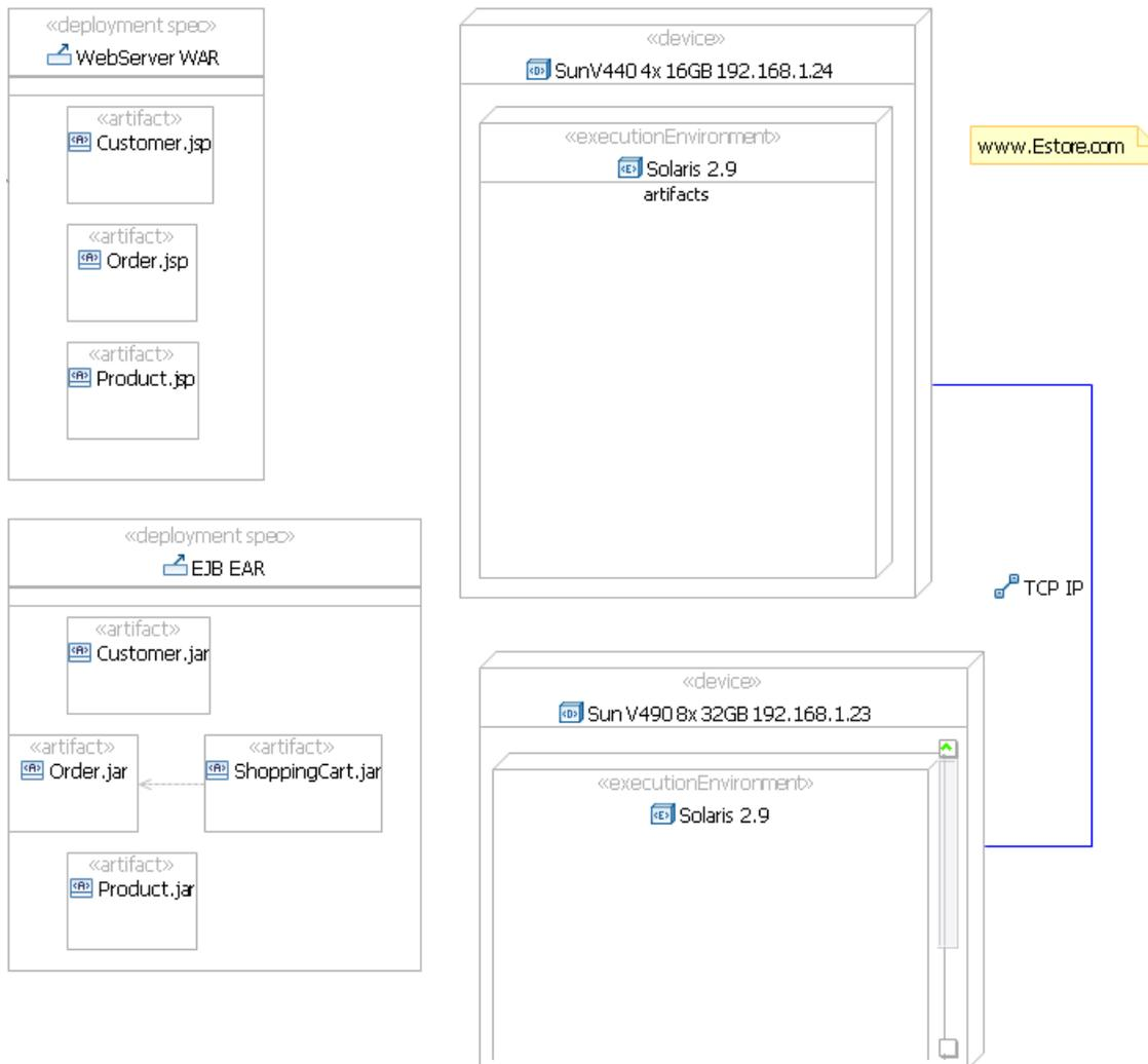
The key elements used in a deployment diagram are nodes, components, and associations. There are two standard stereotypes for nodes: Devices represent physical devices such as a server machine or a workstation, and Environments represent software execution engines such as an Apache Web server, a Tomcat Web container or an Internet Explorer Web browser.
