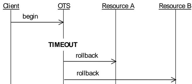
**Figure 6:** *Rollback after a timeout*
