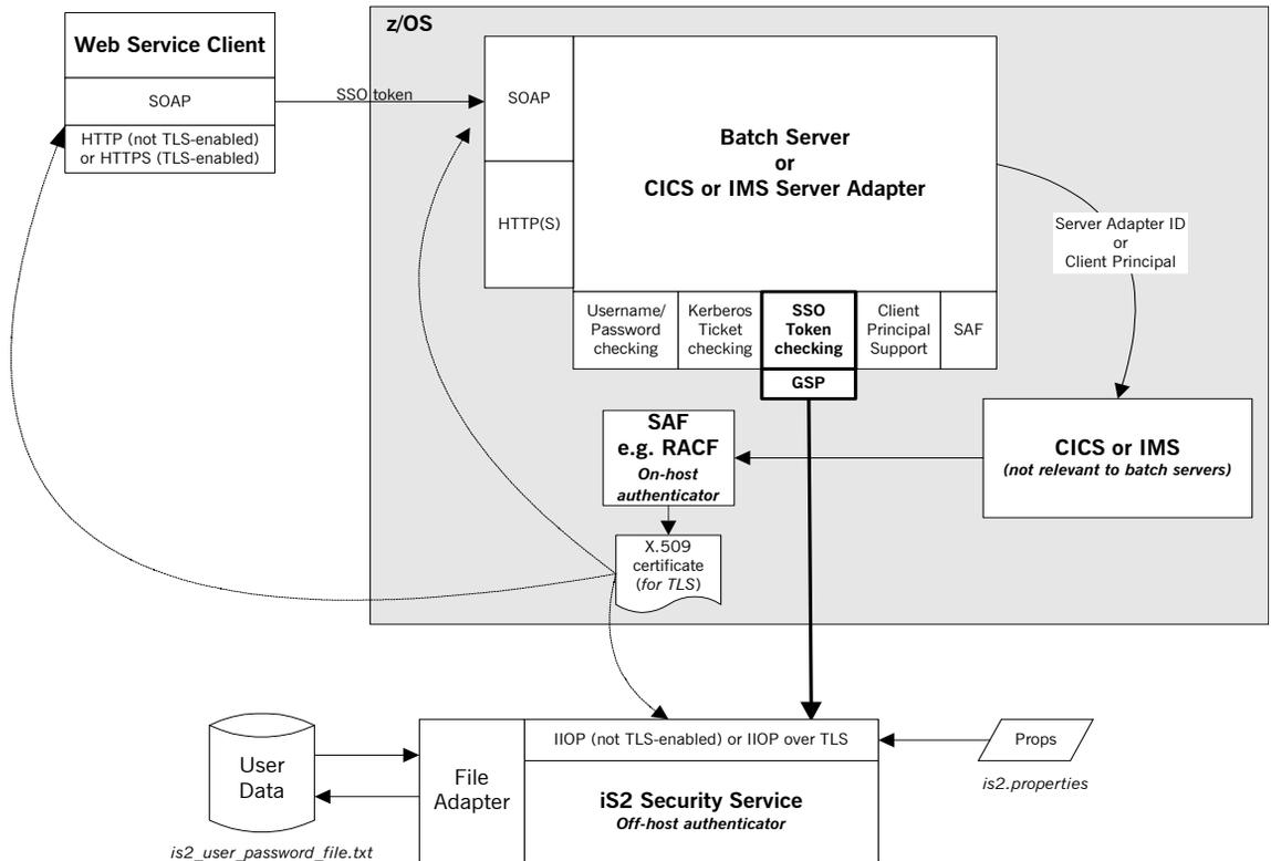
Figure 9: SSO Token Checking in Security Architecture
