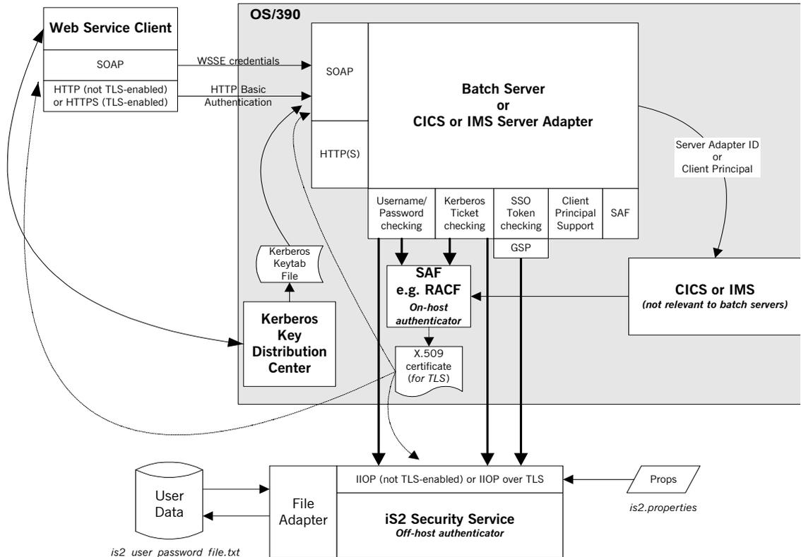
Figure 6: Orbix Mainframe SOAP Mode Security Architecture
