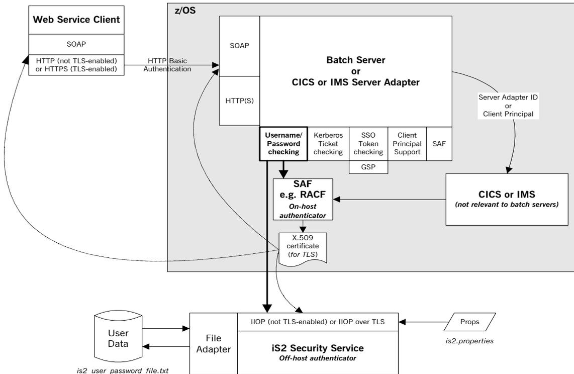
Figure 11: HTTP Basic Authentication in Security Architecture
