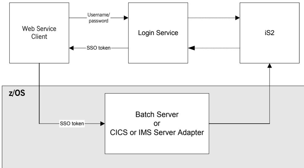
**Figure 10:** Request for and Propagation of SSO tokens
