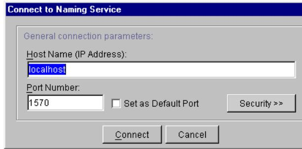
**Figure 17:** Connecting to an OrbixNames Server
