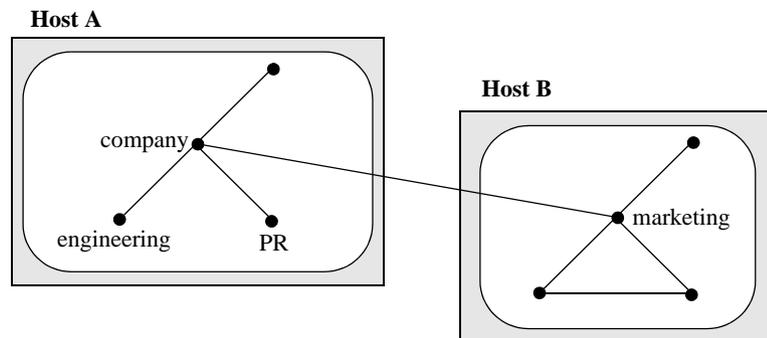
**Figure 8:** Naming Graph Spanning Two OrbixNames Servers
