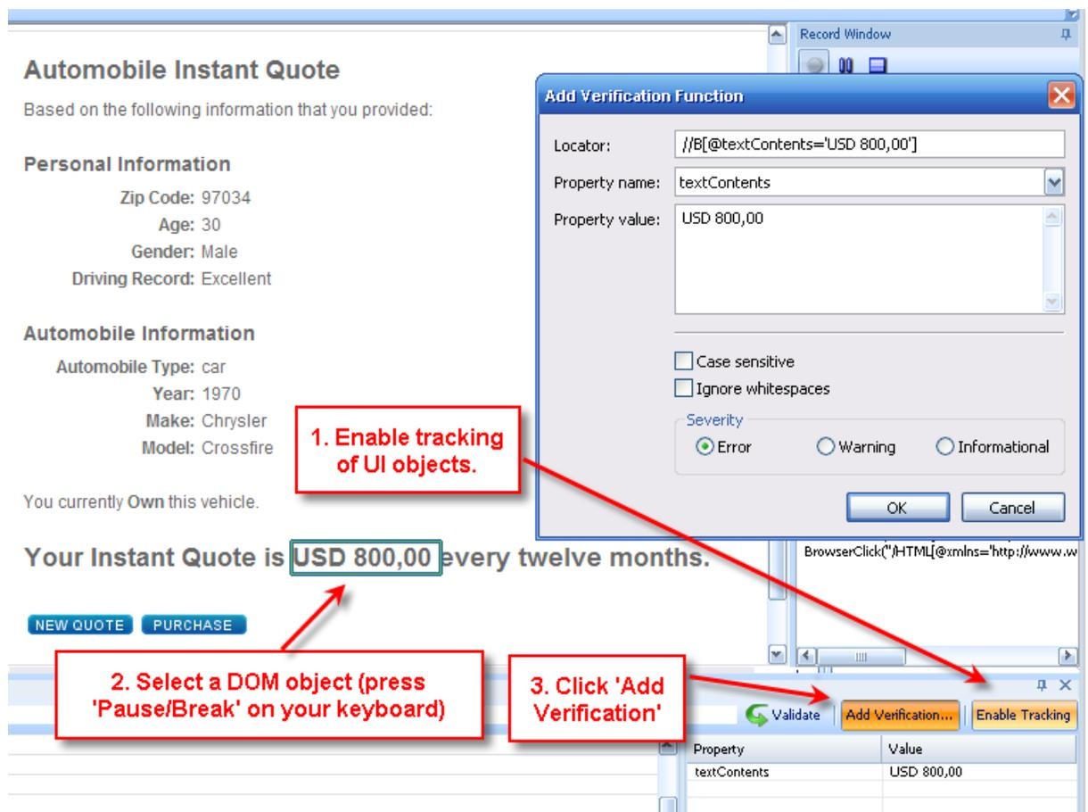
The verification action is recorded in the **Record Window** and the verification function is inserted into the BDL script.
